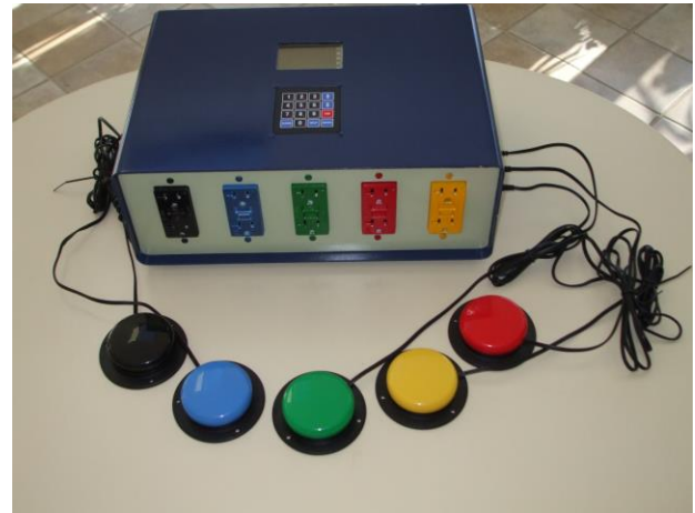
Fig. 16.33. Microprocessor Controlled Power Splitter (MCPS).
