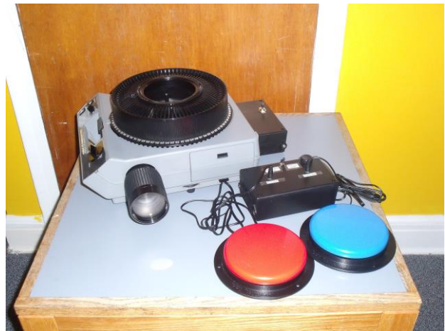
Fig. 16.18. Wireless Switch Activated Slide Projector.
